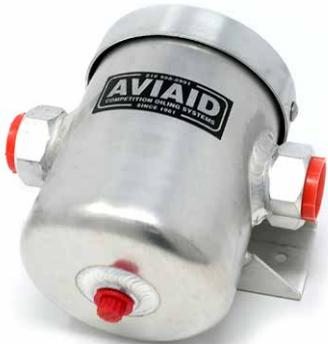
In addition to manufacturing a complete line of dry sump tanks that range in capacities from 1 to 3 gallons, Aviaid makes a compact 1-quart tank that can be mounted near the engine. It measures 5" in diameter and also 5" in depth. There is internal reversing baffling and foam filler. It has two AN-12 female ports and a 3/8" NPT female drain plug bung.
