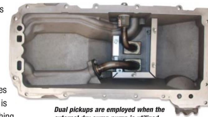
*Dual pickups are employed when the external dry sump pump is utilized*
