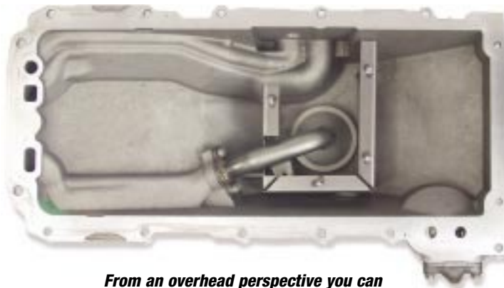
The "cage" insert with trap doors (left) and windage tray provide much-needed oil control for stock LS7 oil pans
