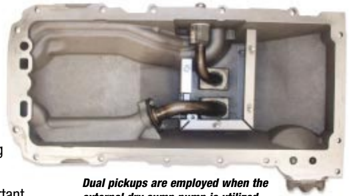
Kit includes pump, idler/drive, belt, 2 pickups and 3 bungs (not shown).
