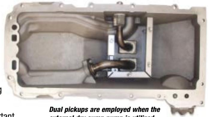
*Dual pickups are employed when the external dry sump pump is utilized*
