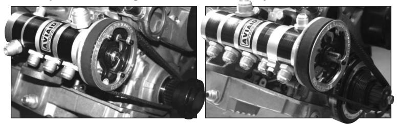
Mounting an oil pump is a difficult enough process without having to deal with the ubiquitous "Big Block Chevy" or a "Small Block Chevy" mount. Aviaid seeks to provide another universal mechanism that allows mounting of custom pumps to a wide variety of engines with the ease and flexibility necessary in today's engine packaging environment. Aviaid's #39 blade mount incorporates a 10mm pivot bore in either the upper or lower corner of the pump.
